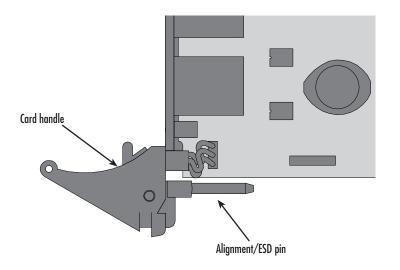
Figure 6. Alignment/ESD pin and card handle
